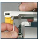
3. Whilst the tool-free blade change control (12) is pressed down the blade to be replaced is free and can be easily removed by using your other hand.
